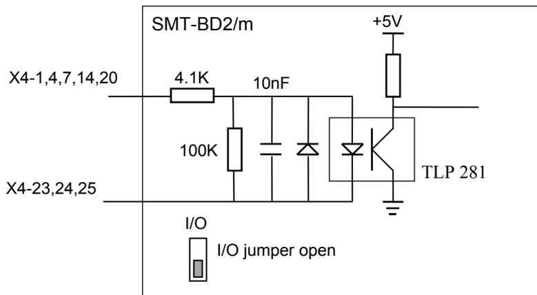
When the I/O jumper is open, the 0 V of the optoisolated inputs (X4 pins 23,24,25) is not connected to the 0 V of the SMT-BD2/m amplifier module (X4, pin 12).
