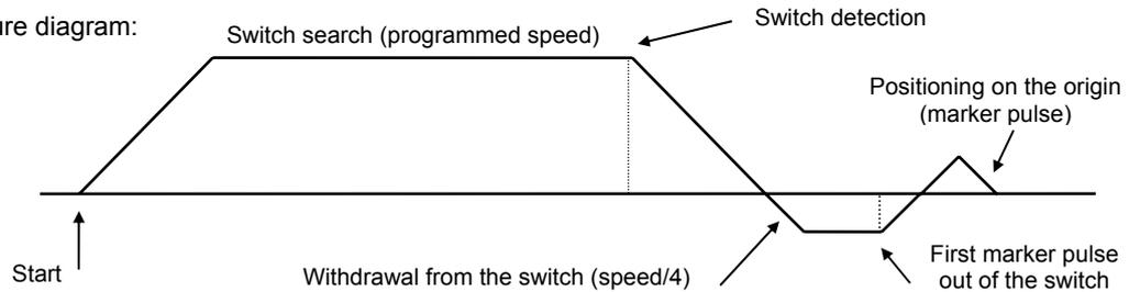
If Switch=1 and Zero=1 or Origin=1, the speed can be reversed by the switch detection or by a limit switch.
