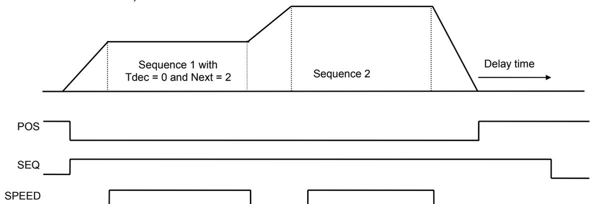
**OUT1 to OUT8** Programmable logic outputs. These outputs are only operating during a programmed sequence.
