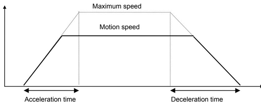
Remark : The JOG deceleration time parameter value is also used when the STOP input is activated.
