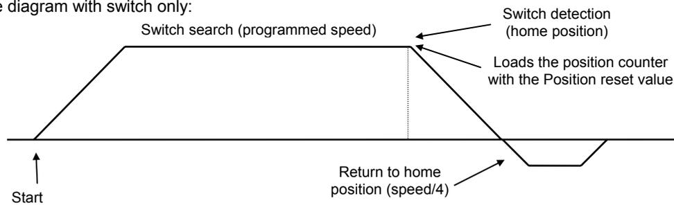
When the sequence 0 contains a homing procedure, at power on, no other sequence can be executed before sequence 0.
