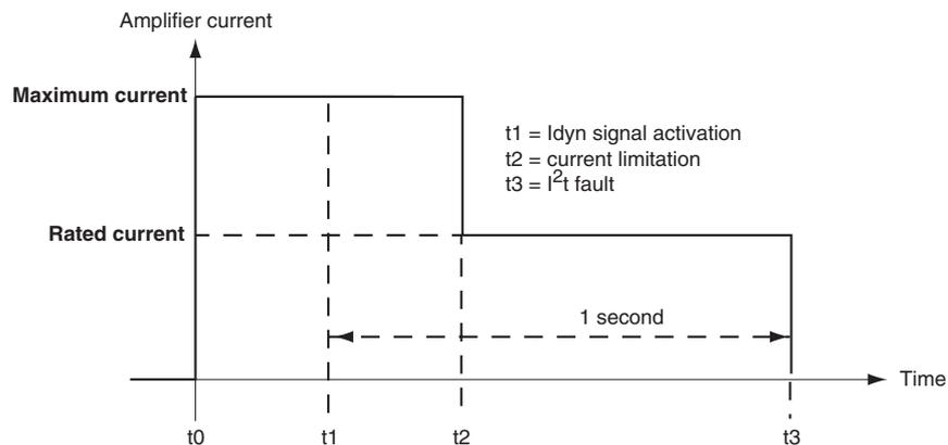
The maximum current duration before the release of the Idyn signal depends on the value of the **Rated current** and **Maximum current** parameters. This value is calculated as follows:
