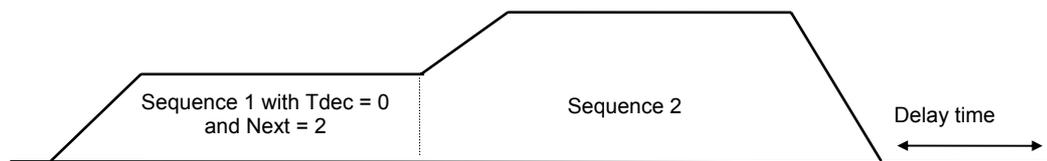
Remark : For a small displacement, when the programmed motion speed value cannot be reached, the trajectory acceleration and deceleration are reduced and the profile is calculated according to the programmed acceleration and deceleration time values.
