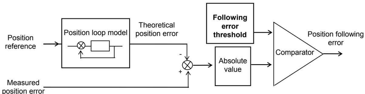
The measured position error is continuously compared with the theoretical position error given by the position loop model. When the difference exceeds the **following error threshold** value, the position following error is released. This following error detection scheme allows to adjust the **following error threshold** to a minimum value when a very sensitive following error detection is required for safety reasons.
