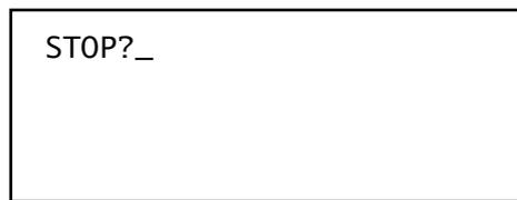
The user must press the
