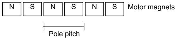
$$\text{Motor encoder resolution} = 1000 \times \frac{\text{Motor pole pitch (mm)}}{\text{Encoder signal pitch (\mu m)}}$$
