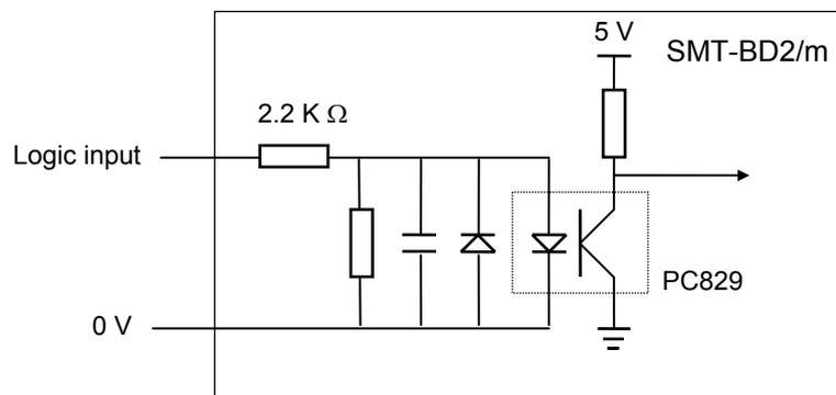
The polarity of these inputs can be reversed by a software parameter. The input voltage corresponding to level 1 is between 5 V and 24 V.
