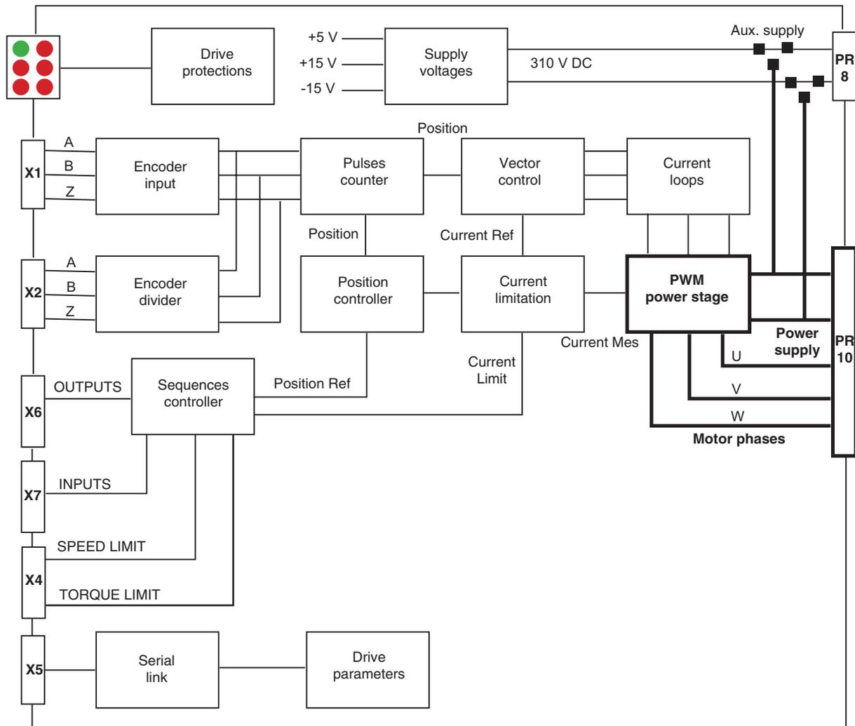
The PR8 and PR10 connectors are not accessible for direct wiring; they are plugged on the BM20A single-axis rack or on the multi-axis BF rack according to the SMT-BD2/m amplifier housing (see chapter 3).
