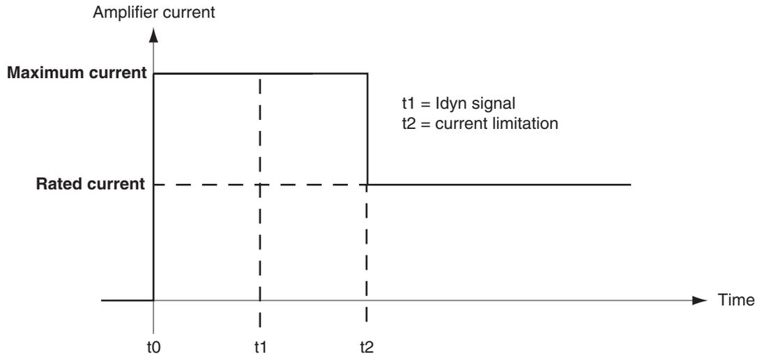
The maximum current duration before the release of the  $I_{dyn}$  signal output ( $t_1 - t_0$ ) and before limitation at the rated current ( $t_2 - t_0$ ) is calculated the same way as for the **Fusing** mode.
