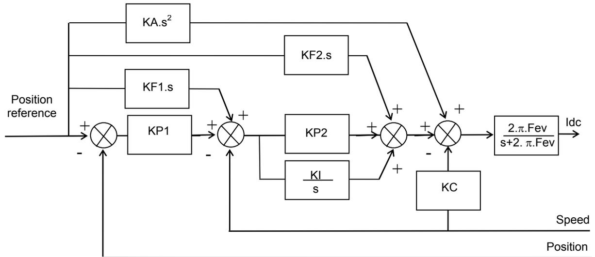
Speed error low-pass filter ( $F_{ev}$ ): defines the cut-off frequency at -3dB of the first order filter which acts on the current command ( $I_{dc}$ ). This value is calculated by the amplifier during the auto tuning procedure and depends on the selected bandwidth and the selected filter type.
