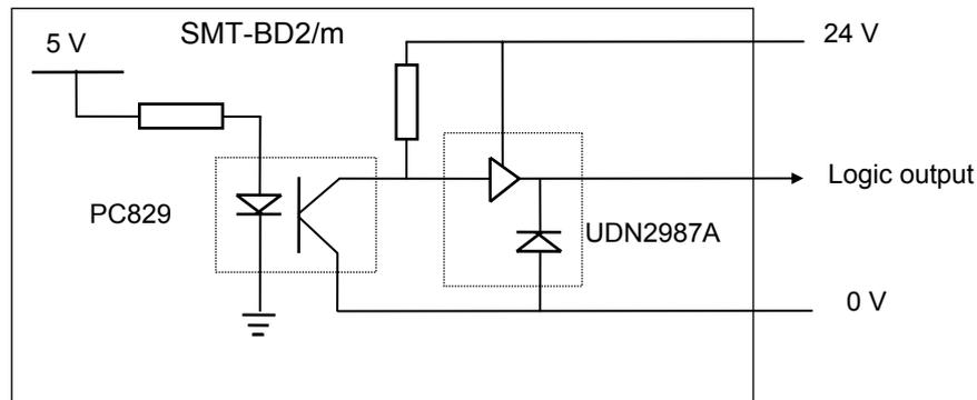
The polarity of these outputs can be reversed by a software parameter. The parallel connection of these outputs must be made by means of diodes. The total output current is 350 mA for the 8 outputs OUT1 to OUT8.
