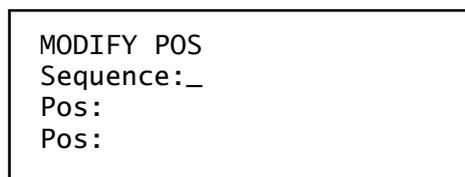
The former position is displayed, and the operator can then enter a new position or cancel by pressing only the ENTER key.
