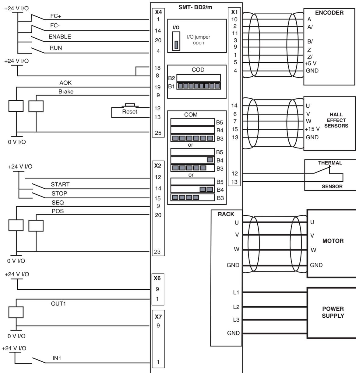
The I/O jumper must be open for getting the X4 connector I/Os optoisolation : the I/O 0 V (X4, pins 23, 24, 25) is disconnected from the 0 V of the SMT-BD2/m amplifier module.
