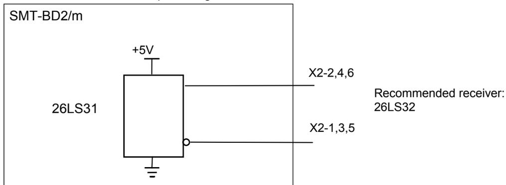
The specifications of the logic I/Os are given in [sections 6 and 7](#).
