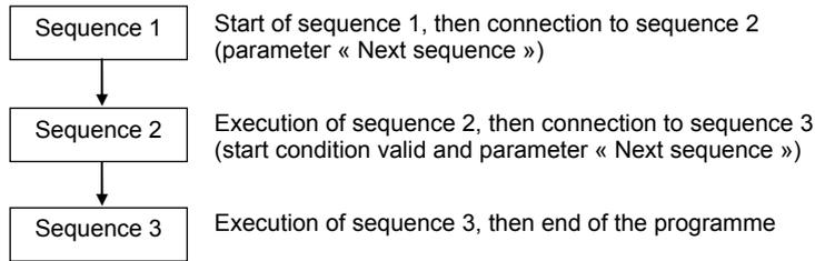
If the execution is starting at sequence 1 and logic input 8 is deactivated, the programme will be the following:
