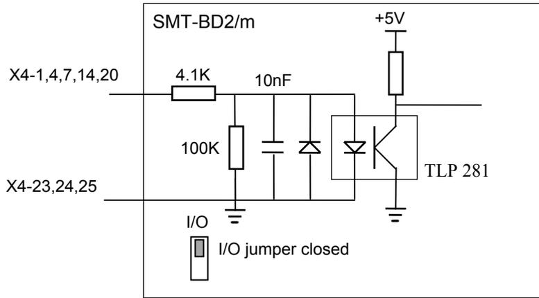
When the I/O jumper is closed, the 0 V of the optoisolated inputs (X4, pins 23, 24, 25) is connected to the 0 V of the SMT-BD2/m amplifier module (X4, pin 12).
