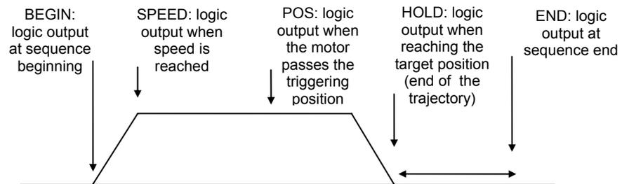
In a homing sequence, the outputs trigger only at the end of the sequence.
